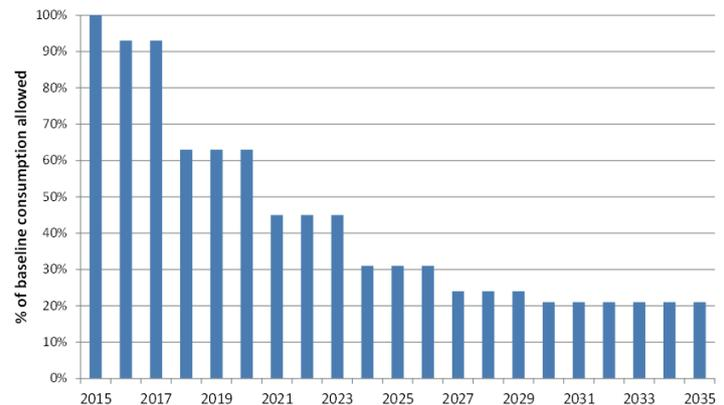
From 2018 onwards, the EU F-Gas Regulation [EU 517/2014] creates massive cuts in the consumption of HFCs in the EU. This reduction scheme, known as the HFC phase-down, is based on a quota system. Quotas are expressed in CO<sub>2</sub> equivalent (kg x GWP).
