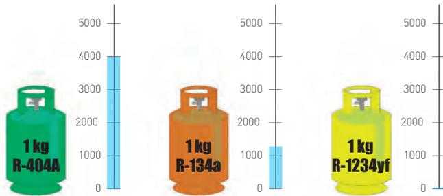
The higher the GWP of a refrigerant, the more it will come under pressure by the HFC phase-down, even though the phase-down does not prohibit any refrigerants.
